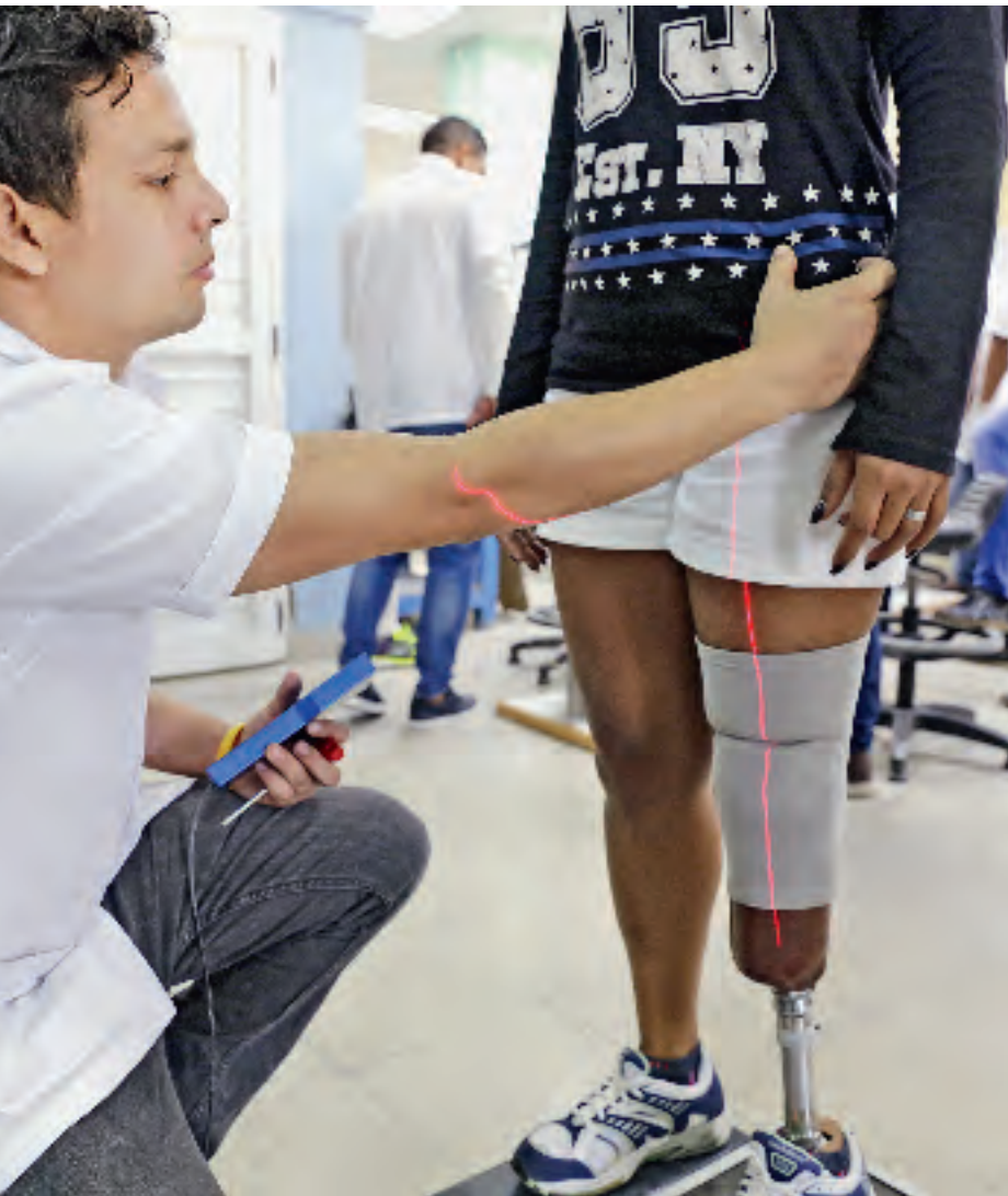
Technician Eriel Castillo works with a new laser measuring device to ensure that his prostheses sit perfectly.
