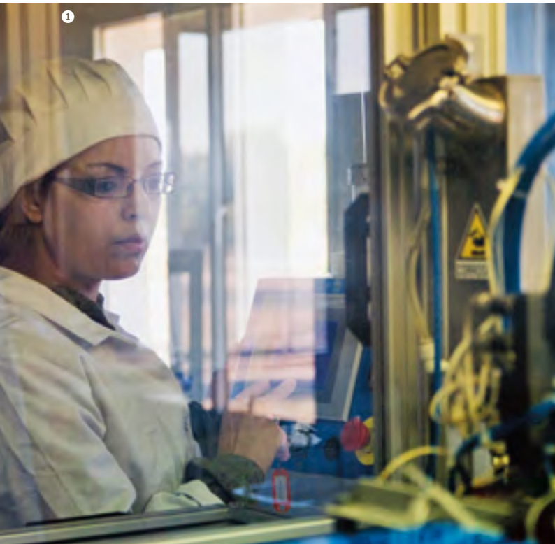
❶ A local worker uses a stringer machine to interconnect solar cells. ❷ A primary school near Ifrane has a power plant on its roof. ❸ A wind farm near Essaouira
